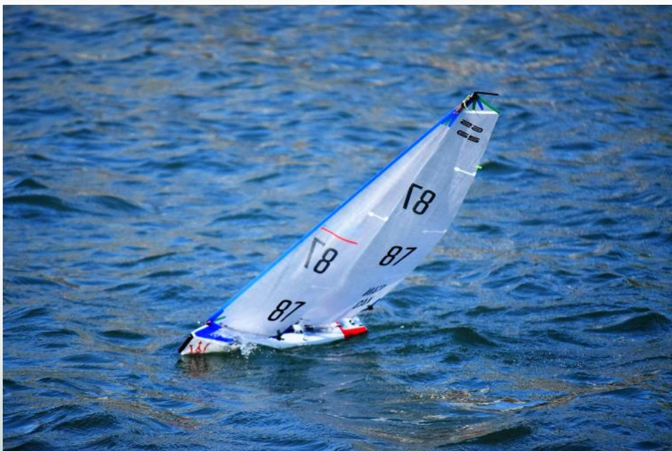
The A+ rig on the DF65 is a masthead rig, just like it's bigger brother the DF95
