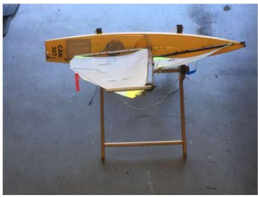
difference is some ram – note how the leach has closed towards the backstay around area of the orange wind telltale. This is exaggerated as shown, as there is no wind pressure on the sails.
