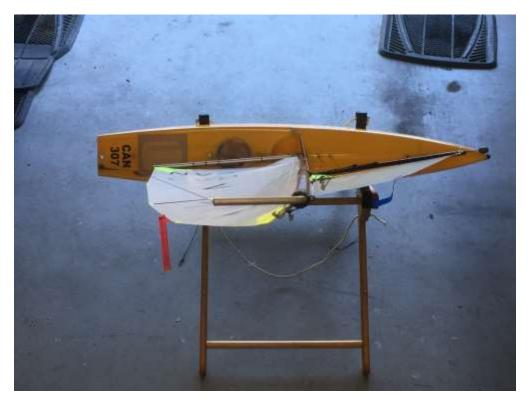
Next set the mainsail twist by adding mast ram to push the bottom of mast into column. This pushes the top of the mast up and closes the mainsail leach. To see the effect, hold the boat up and push aft on the mast at the mast ram, while watching the mainsail upper leach open and close as you push and release. This is what the ram is all about.
